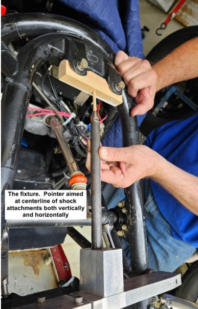
Fixture is loaded with the new pins and being pointed in order to obtain the correct angles
