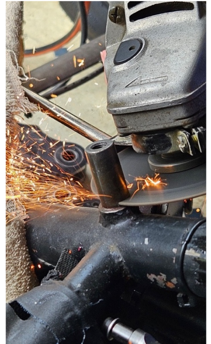
Cutting off the old pins. I was kinda anxious at this point!
