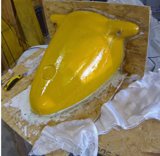
Plug with 1 st Layer of Fiberglass Applied
