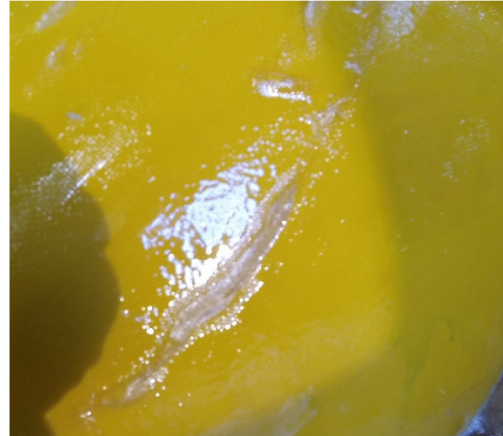
Plug with 1 st Layer of Fiberglass Applied
