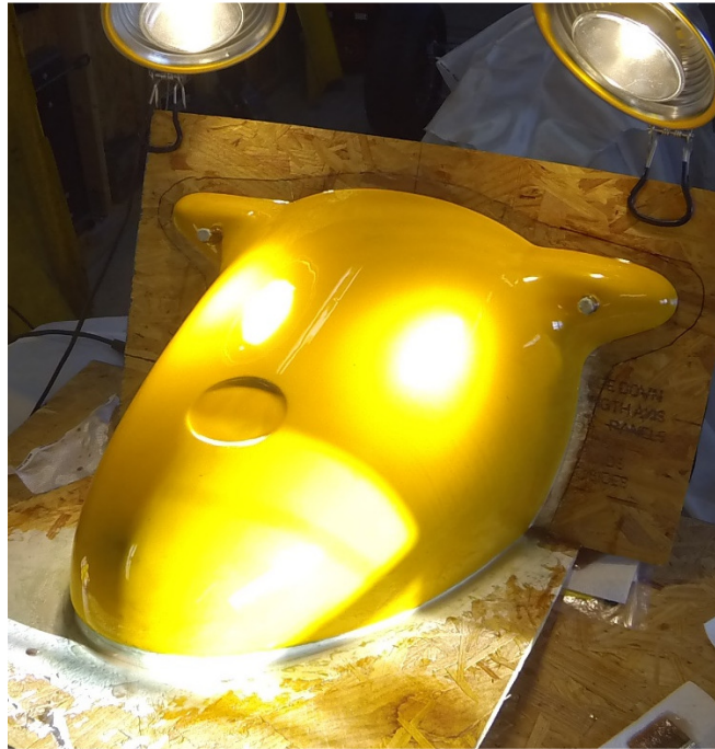
Plug with 1 st Layer of Polyester Applied
