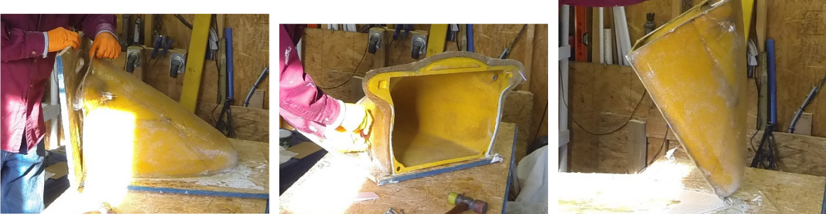
Removing the Fiberboard Base Plates
