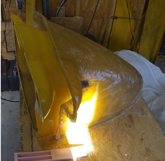
The Plug is Released from the Mold
