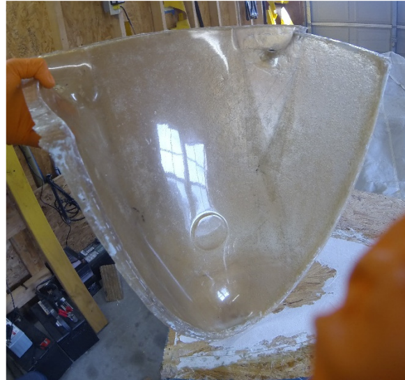
The Plug is Released from the Mold
