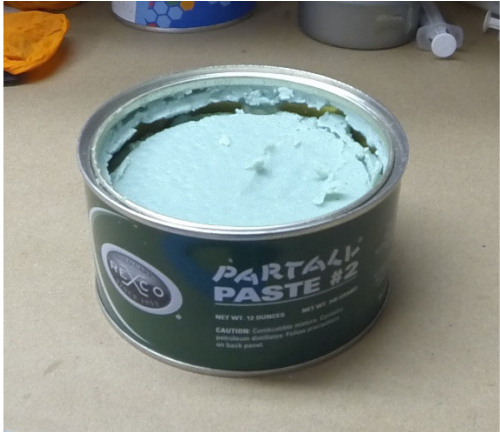
Parting Wax and Polyvinyl Alcohol (PVA)
