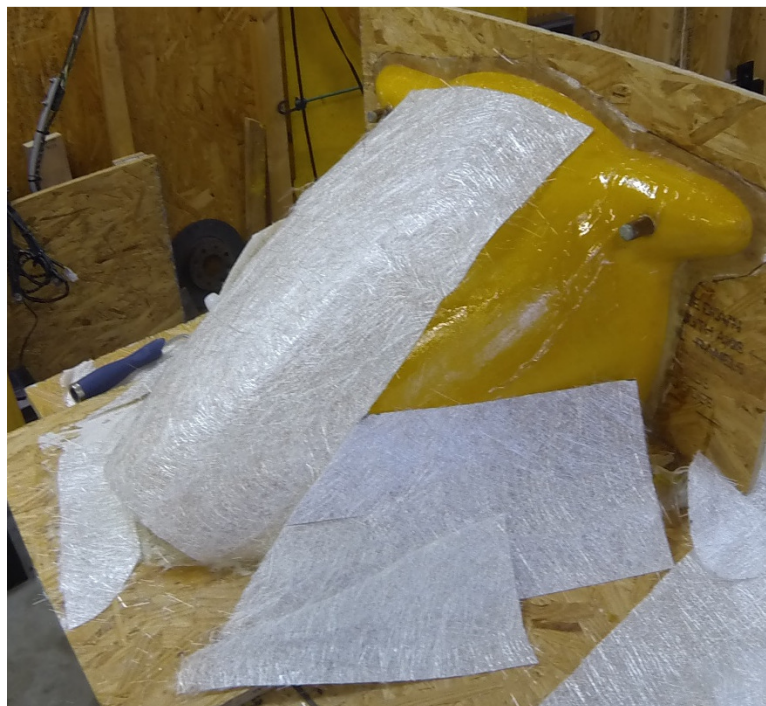
Plug with Various Pieces Layed out for Fitting
