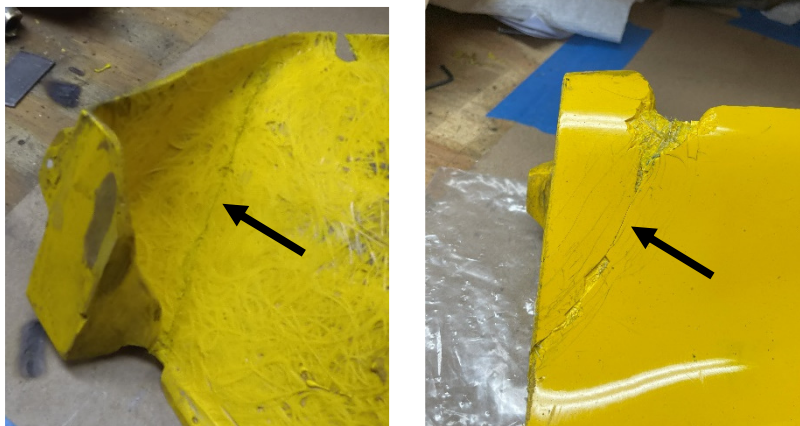
Crack On the Inside and Outside
